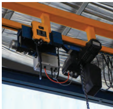
Hoist Trolley Drive with remote control receiver
