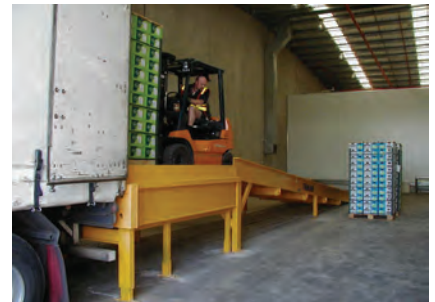
Ramp and Dock Leveller combination
