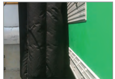
Eco Shelter inflates to seal flush against the trailer
