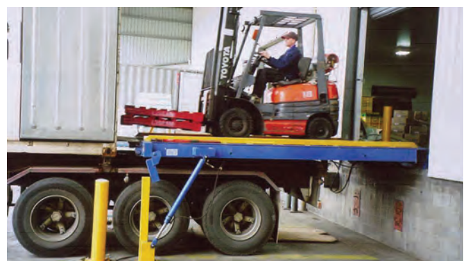
Safetech Hydraulic Container Dock Leveller (model CDL) designed to allow container truck trays / "B" Doubles to back under for safe loading and unloading
