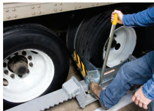
Manual Wheel Chock – where securing a trailer's rear impact guard is not an option
