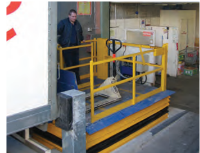
Safetech Scissor Hoist for loading docks that are not raised
