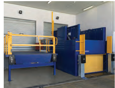
Safetech Low Profile Rail Hoists need no pit and can complement the function of typical loading dock levellers
