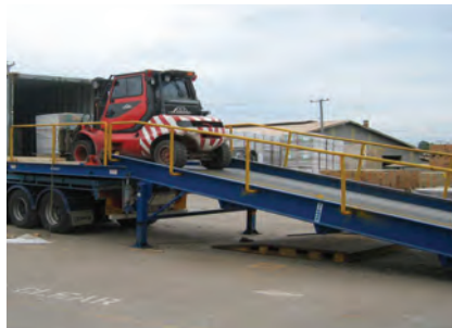
Conventional Container Ramp
