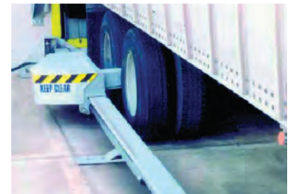
Effective vehicle wheel chocking – prevents trailer creep and premature departure
